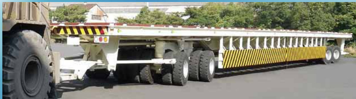
200t 200t TT 台車 200-ton TT specialized full-trailer
