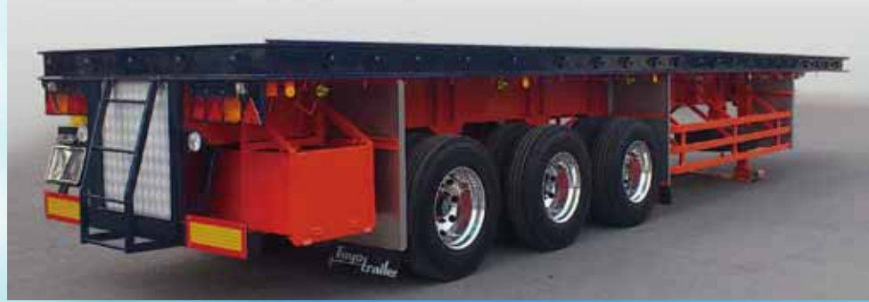
200t 200t TT 台車 200-ton TT specialized full-trailer
